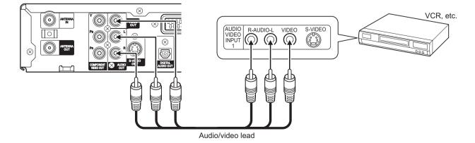
When connecting a VCR, etc. having an S-video terminal, connect by an S-video lead.
